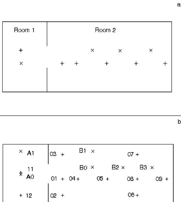
FIG. 2. Two-room coupled system. Transverse section (a) and plan (b) views are shown. The volumes  $V$  and areas  $S$  of the subrooms are  $V_1 = 6270 \text{ m}^3$ ,  $S_1 = 2066 \text{ m}^2$  (15 m × 19 m × 22 m) and  $V_2 = 17\,556 \text{ m}^3$ ,  $S_2 = 4280 \text{ m}^2$  (42 m × 19 m × 22 m) and; areas include coupling areas. Crosses (+) indicate receiver positions: 1–9 in Room 2, 11–14 in Room 1. Sources are indicated by X's: A0-A1 in Room 1 and B0-B3 in Room 2.
