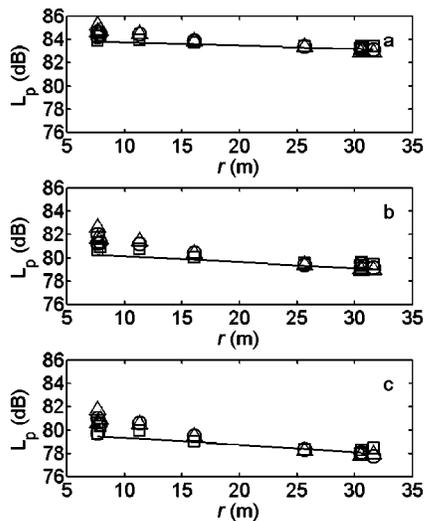
FIG. 5. Sound propagation curves (with direct sound subtracted) in Room 2 for Source B3 and  $S_{12}=25\text{ m}^2$  in Conditions 1 (a), 2 (b), and 3 (c) computed by the GA model for  $s=0.10$  (squares),  $0.60$  (circles), and  $0.99$  (triangles) are compared with the predictions of Eq. (16) (solid line).
