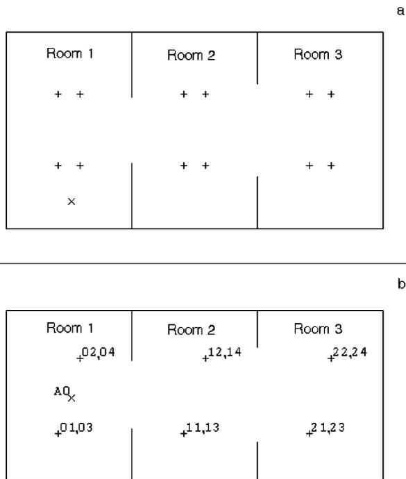
FIG. 1. Three-room coupled system first studied by Kuttruff. Transverse section (a) and plan (b) views are shown. Volumes  $V$  and areas  $S$  are the same for each subroom:  $V=6270 \text{ m}^3$  and  $S=2066 \text{ m}^2$   $15 \text{ m} \times 19 \text{ m} \times 22 \text{ m}$ ; areas include coupling areas. Crosses (+) indicate receiver positions: 1–4 in Room 1, 11–14 in Room 2, and 21–24 in Room 3. The single source position in Room 1, A0, is indicated by an X.
