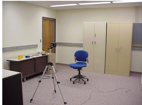
Fig. 1. The measurement room environment (5.7 × 4.3 × 2.6 m). The loudspeaker sound source, and seated listener location are also shown.
