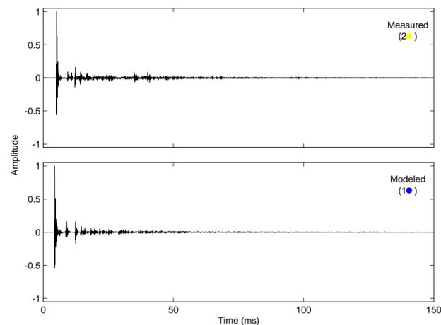
Fig. 2. Measured and modeled binaural room impulse responses (BRIRs) for listener SZI. Only the first 150 ms of the responses from the left ear are displayed.
