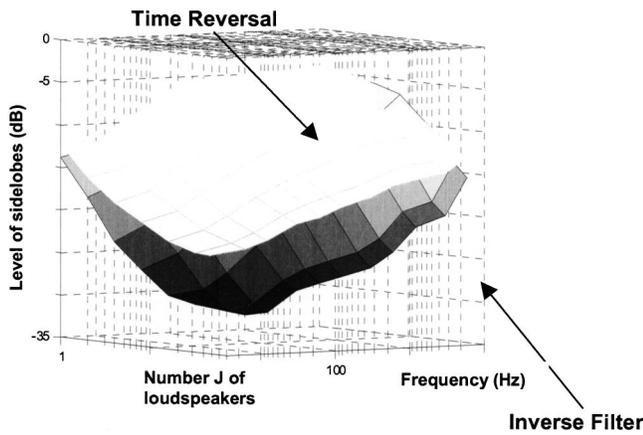
FIG. 6. Evolution of spatial sidelobe level  $SL_{(dB)}$  as a function of the number of used transducers  $J$  and of the bandwidth  $BW$ , for time reversal and inverse filtering. Measurements are averaged over 16 repetitions.
