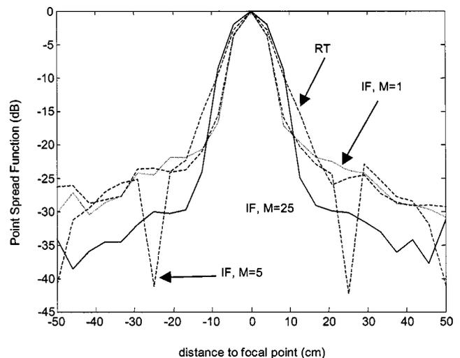
FIG. 5. Directivity patterns obtained with time reversal and inverse filtering for different numbers  $M$  of control points.
