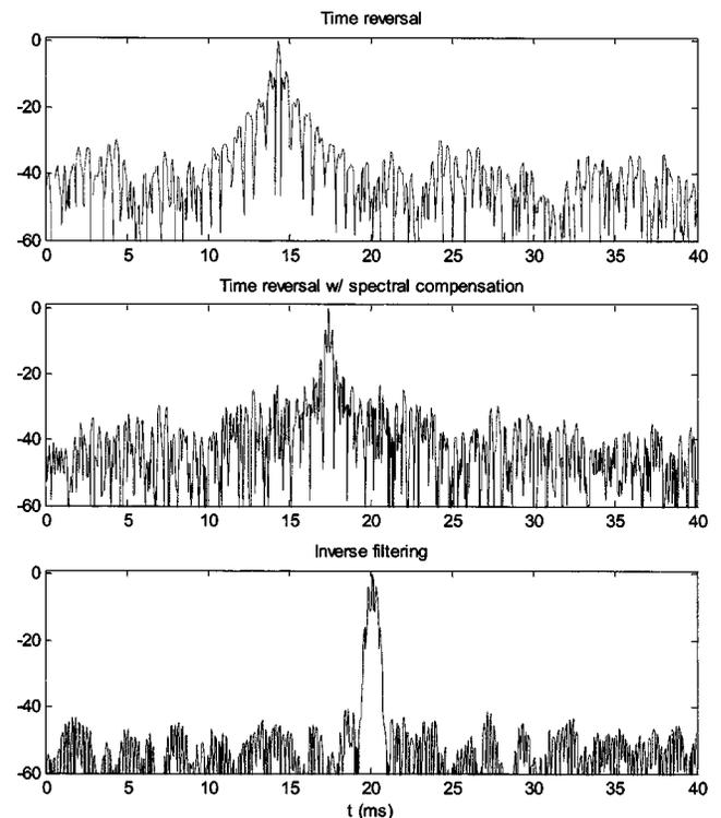
FIG. 8. Temporal sidelobes and temporal recompression observed at the focal spot, for the different techniques. The signal amplitude is presented in a dB scale.
