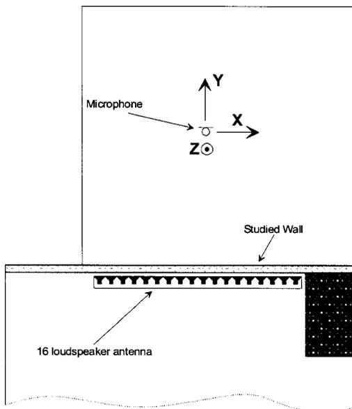
FIG. 11. Experimental setup for focusing through a wall.
