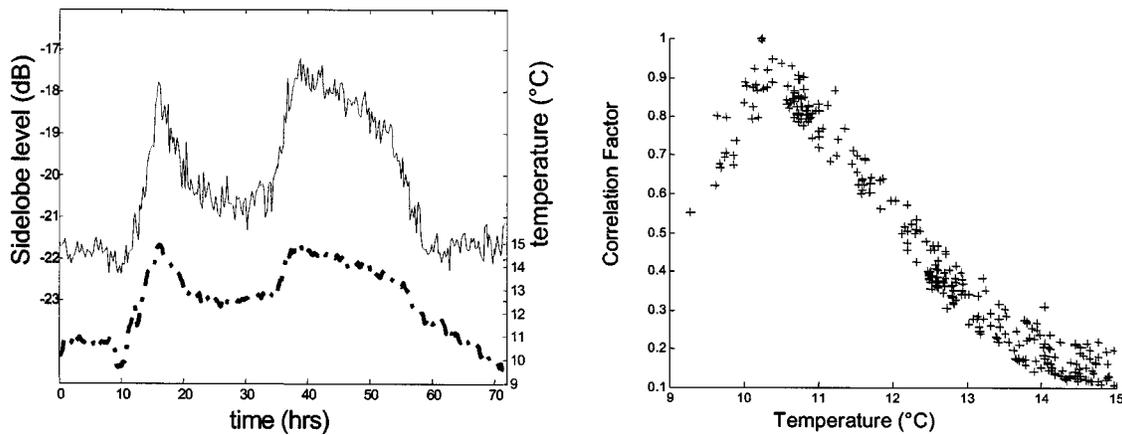
FIG. 9. Robustness of focusing versus temperature and time: initial time  $t=0$  corresponds to the acquisition of the propagation operator. The solid line corresponds to the evolution of the level of the sidelobes while focusing every 15 min at the same focus location. The dashed line corresponds to the evolution of temperature operating at the same time.
